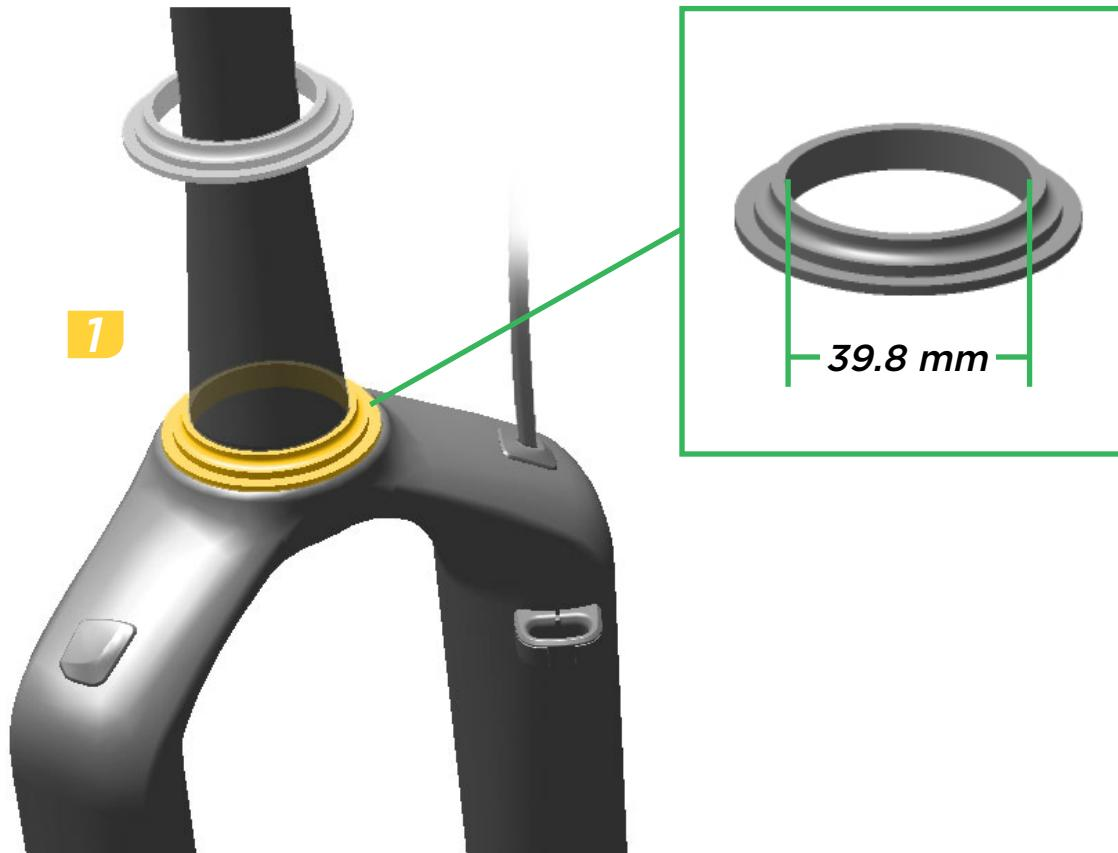
Install a headset into the bicycle frame and a crown race onto the fork according to the headset manufacturer's instructions.
