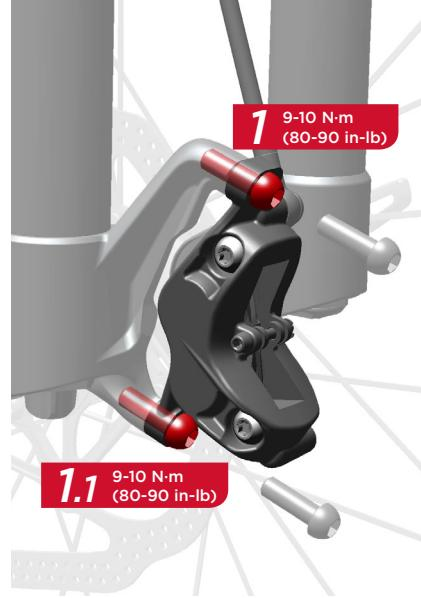
Adjust the hose angle to prevent the hose from rubbing against the fork, if possible.
