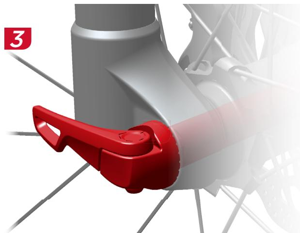
Lever tension is sufficient if the lever leaves an imprint on your hand. To increase lever tension, open the lever and turn it clockwise. Close the lever to recheck lever tension. Repeat until the tension is sufficient, then close the lever. When the lever is closed, verify there is no gap between the lever head and dropout.
