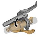
5. Secure the clamp band of the brake lever. Secure the lever using the fixing screw.
