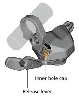
3. Replace the inner cable and slide the inner hole cap closed.
